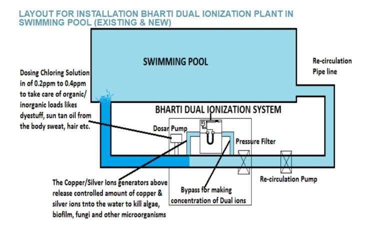
Every swimming pool will have a recirculation system comprising of pressure sand filters, pumps etc which will be housed inside a room. We can fix the equipment inside this room and can take by pass connection from the outlet of the filter and connect it to the pool. The control panel has indications to show that electrode is working, electrode needs cleaning, electrode is worn out. It also has the provision to increase or decrease the dosage
