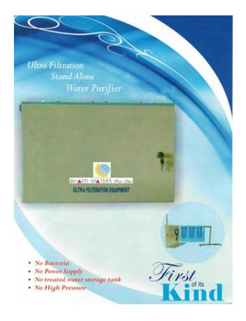
This state of art membrane filters particles of the size of 0.01 micron and above. So this filters the turbidity, Iron content and all bacteria from water. This capacity of bacterial filtration is guaranteed through out the life of the membrane. As all the bacteria are filtered, no separate disinfection equipment is required.
